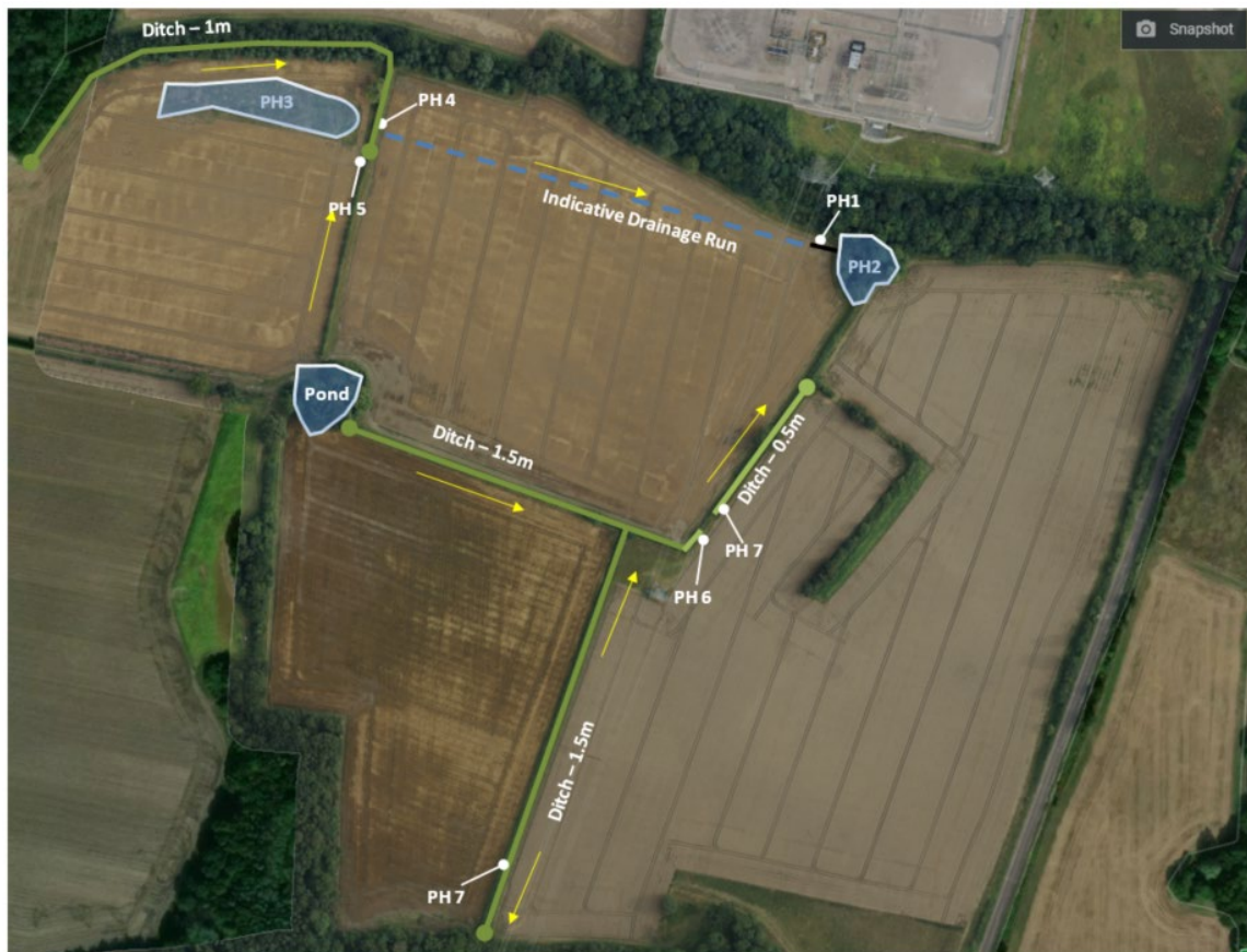
Figure 6: Ditches and Hollows Local to the Onshore Substation Site
